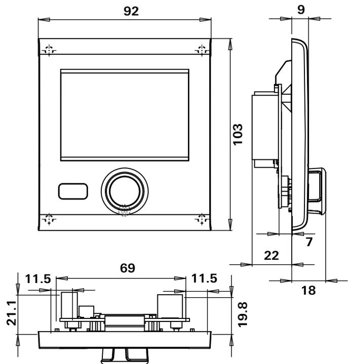
Fig. 18 – Dimensions in mm. Picture not to scale
