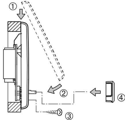
**Fig. 22** – Installing the control panel upper part and rotary push button
