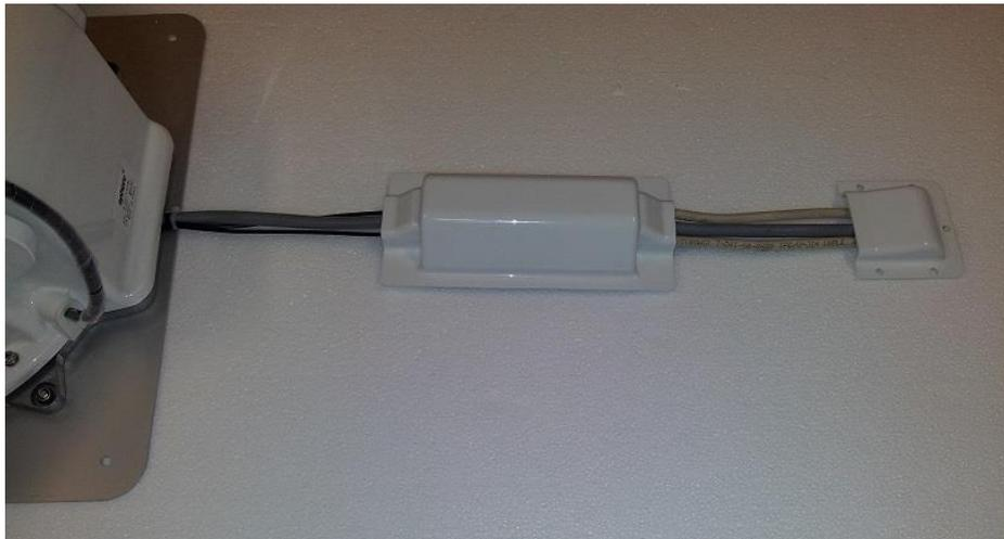
Example of cable cover and entry plate ready to be glued and screwed into position.
