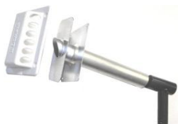
LS300 vent and frame cut out required 490mm x 249mm. Each vent has open area of 667 cm 2
